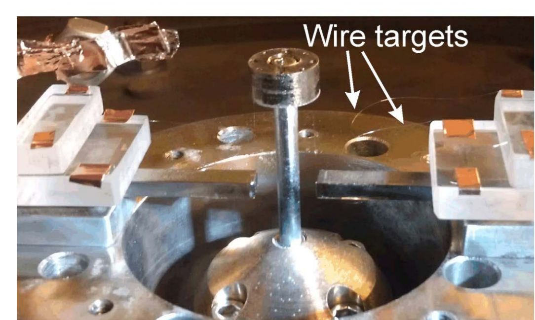
Figure 1: Photograph of the experimental setup on Cornell's XP machine (150ns, 300kA)
