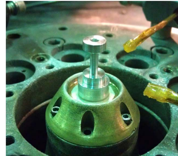
Z-scale liners, aluminum (150 \mu m thick, 3mm OD and 10mm tall)
